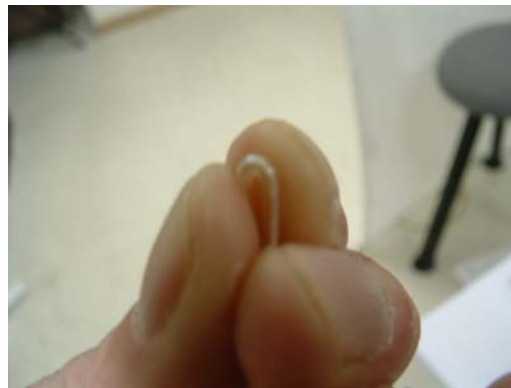
Figure 13. Cable Bent to the Material Limit
