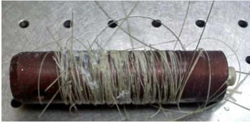
Figure 6. Carbon Fiber Sample with Breaks Along Length
