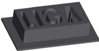
Step 4. Planarize and remove polymer
