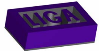
Step 6. Molded polymer part
