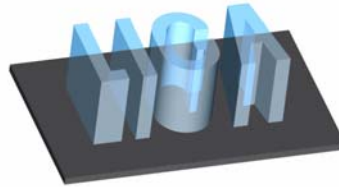
Step 2. Develop Exposed Polymer
