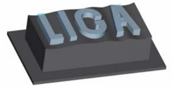
Step 3. Electroplate through exposed areas
