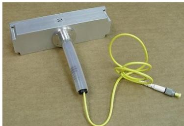
As a standard product for mobile robots we offer a unit that deploys an expendable optical fiber at very low tension. It includes a flexible 'tail' that minimizes the chance the fiber could be damaged when the vehicle backs up or makes tight turns. Produced using a fully-automated, high-precision process we achieve low pack attenuation and low unit cost. Standard configuration is 5.5"x1"x1.5", and is available with fiber lengths of up to 700 m of singlemode fiber.
