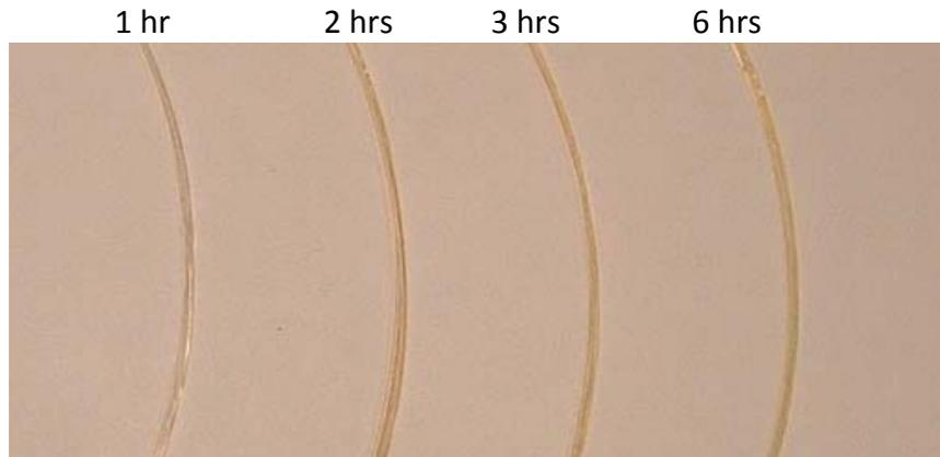
Figure 2. STFOC Fibers After Baking / After Stripping LCP Coating
