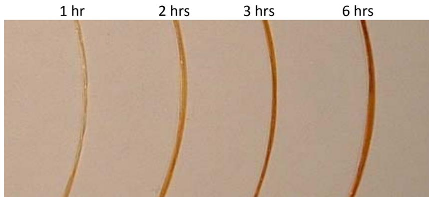
Figure 1. Bare Fibers After Baking
