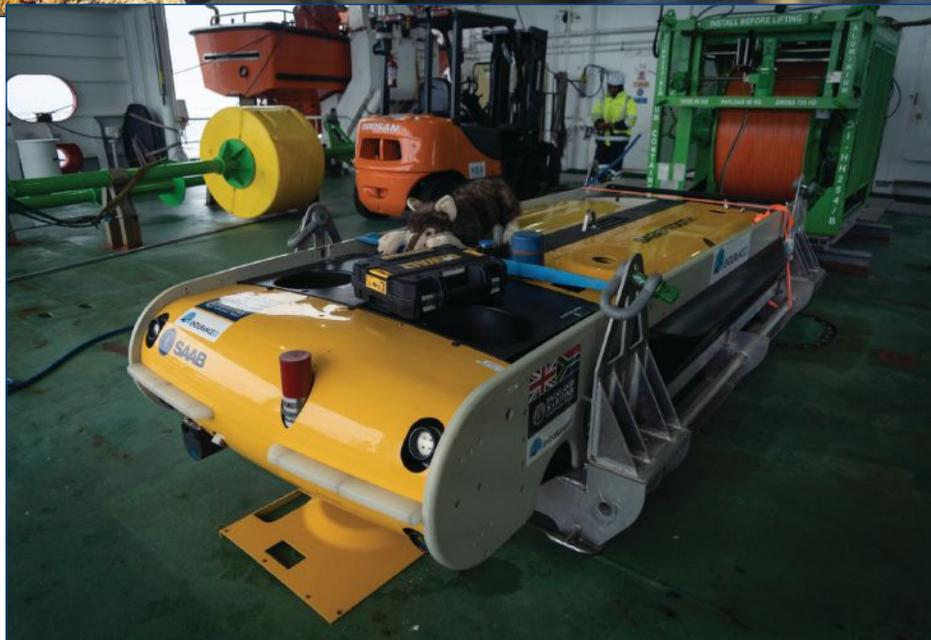
*(Top) Extrusion of low-density outer jacket. (Bottom) LIN-DEN-SPE-7098 attached to Saab Sabertooth ROV. (Credit: Falklands Maritime Heritage Trust)*
